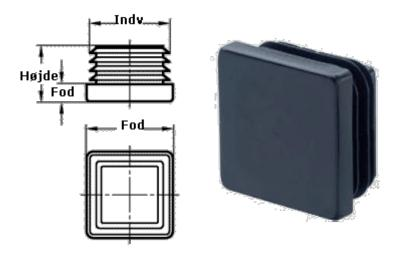
Foot diameter = 50 mmFoot length = 5 mmHeight = 23 mmInternal tube diameter = 46 mm
